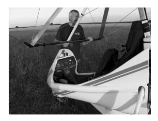
4.4.9. Attach the mast brace tube in to position, bolt it and secure with a nut and a safety ring.
