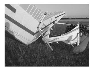
4.4.2. Lift the nose of the wing up until high enough to connect the universal junction of the trike to the U-bracket of the wing. and allow the bushing of the U-bracket of the wing to slide into position into the slits on the universal junction of the trike. Insert the heart bolt, tighten wing nut firmly and secure with a safety ring.
