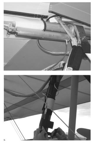
Connect the pin and socket connector of the trim device.
