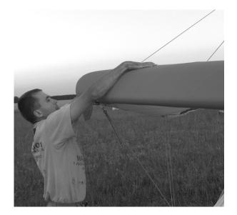
4.4.8 Apply the trike park brake. Go to the nose of the wing. With the mast brace tube in one hand and the control bar in the other hand lift the base tube. Rise the wing up. In strong winds maintain a firm grip on the wing.
