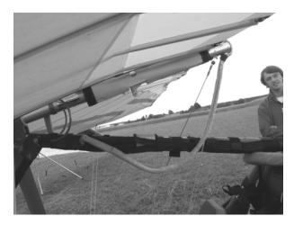
4.4.4.Connect backup loop so that it passes over the keel and back to the pylon. Tighten a nut and secure with a safety ring.
