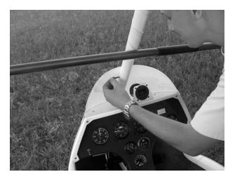
4.4.10.Install the bolt into the pilon's joint as shown on the picture.
