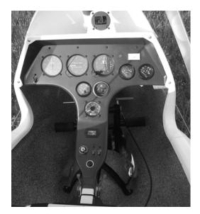
The Pitot static gage supplies ram air pressure to the air speed indicator from the nose of the cockpit. The static pick up is at the rear of the instrument under the dash.
